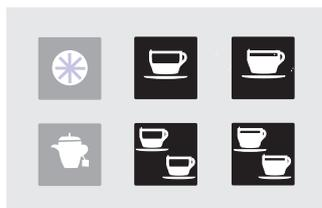
Pushing one of these buttons (key1, key2, key3, key4), if the keyboard is connected with group 1(KEYBOARD1) the output of the group 1 (EV1/PL) is activated for the volume of the programmed dose or if the keyboard is connected with group 2(KEYBOARD2) the output of the group 2 (EV2/PL) is activated for the volume of the programmed dose.
